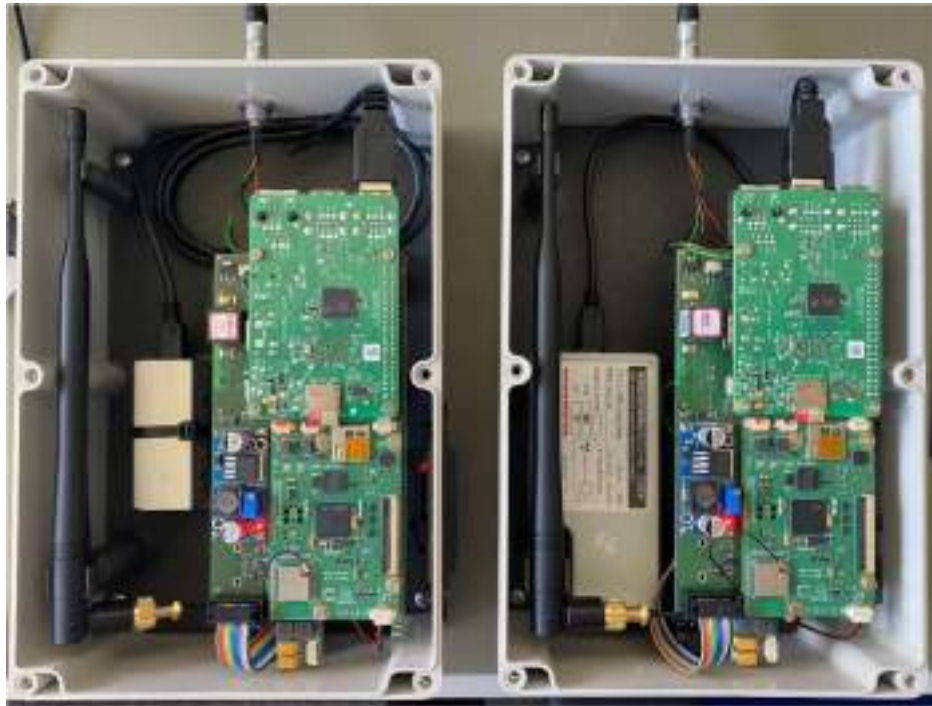
Figure 12 Interior view of the stationary platform of the Sensor Integration Unit (SIU)
