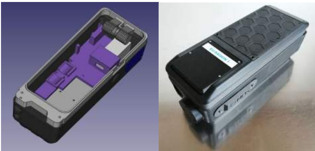
Figure 9 On the left hand side: the CAD model of the portable Sensor Integration Unit (SIU), representing the initial phase in the development of the handheld device; the final design of the handheld SIU is presented on the right panel
