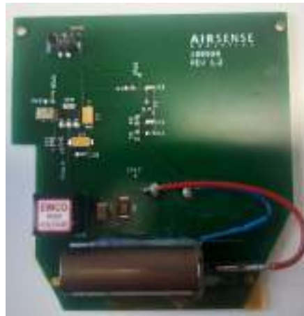
Figure 4 Printed Circuit Board (PCB) featuring the GM Tube and associated electronic components
