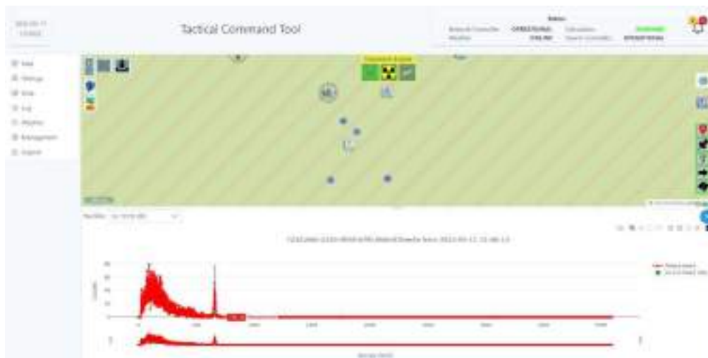
Figure 25 Figure captures the Gamma spectrum of a Cs-137 sample obtained during field trials in Umeå on 05/23, highlighting the UI's efficiency with actual radiological samples.
