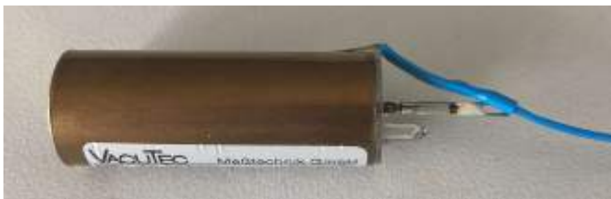
Figure 3 The Geiger-Müller (GM) tube chosen for the EU-RADION project
